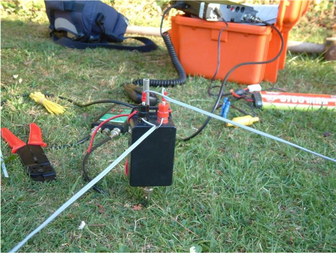
Fig 3 – connection of phasing lines to the 4:1 balun. Phasing is changed between in phase and 180 degrees out of phase simply by reversing the connections of one of the phasing lines. The phasing lines are kept gently taut so that they remain a few inches above the ground, although no deterioration in performance was observed when they were allowed to sit on the ground.
