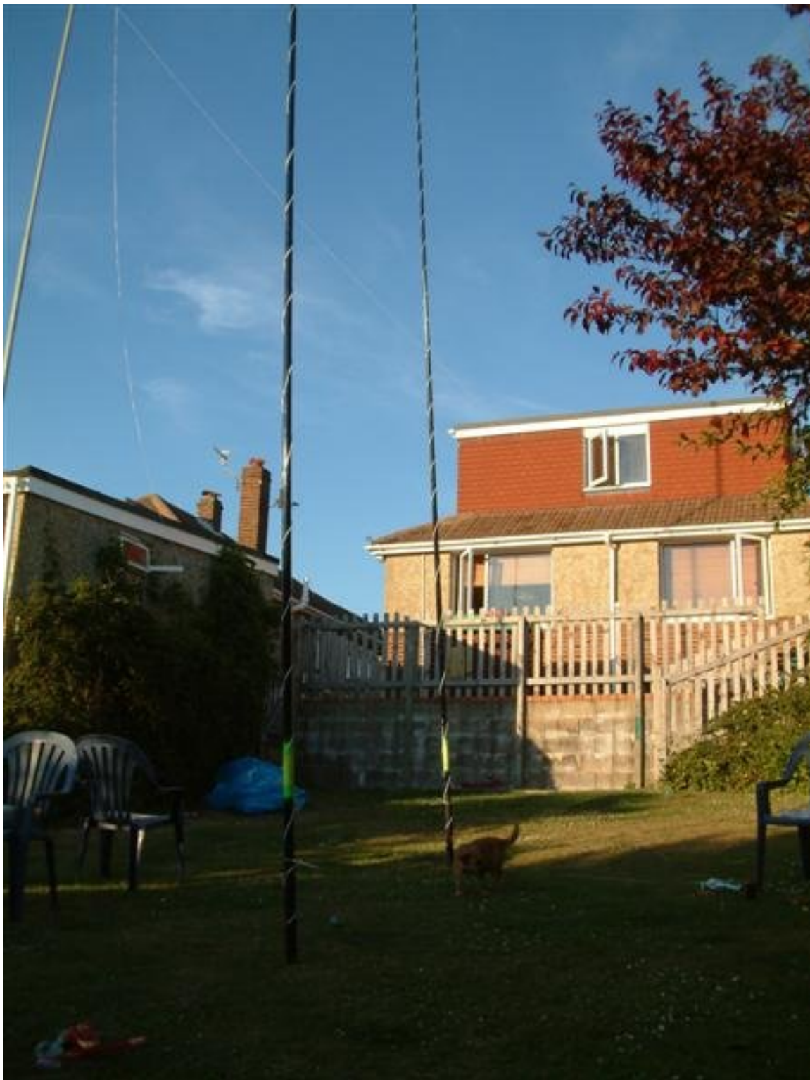
Fig 4 – the “no counterpoise” two elements phased array at Chez M3KXZ. Note the small dog by the furthest antenna – she likes to keep up with whatever is going on. Note also, that each “no counterpoise” antenna is wound helically around the fishing pole for ease of set up and neatness. Such gentle winding should have minimal impact on antenna performance.
